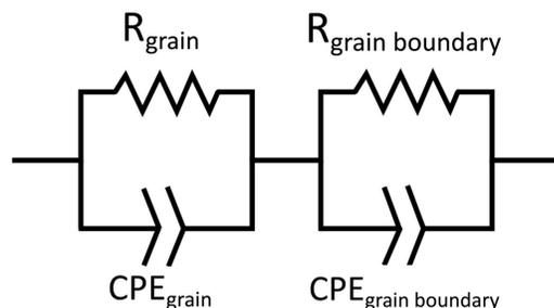
Fig. 2. The EIS equivalent circuit used. Both lattice and grain boundary resistance and capacitance contribute to the AC response. Curve fitting was done in ZView.
