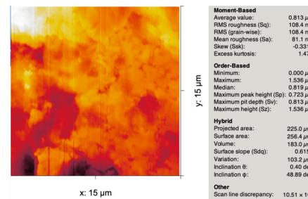
Fig. 4. Sample AFM micrograph of heat-treated pellet surface
