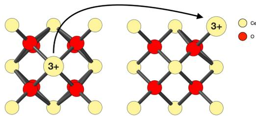
Fig. 1. Small polaron hopping in CeO<sub>2</sub>. (DFT calculations predict that the reduced Ce-O bond length is 0.091 Å longer than the bond length in a perfect crystal) [2].
