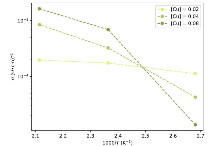
Fig. 5. Arrhenius plot of the three compositions measured.
