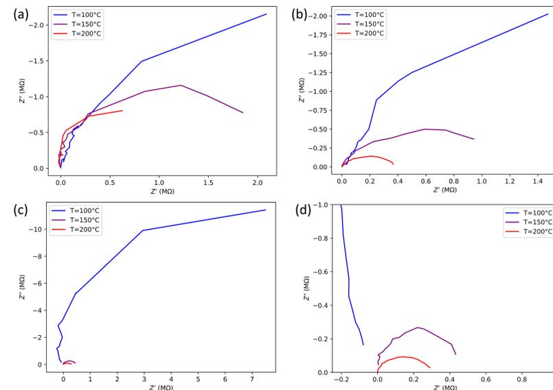
Fig. 3. Nyquist plots for (a), 2% Cu doping, (b), 4% Cu doping, (c), 8% Cu doping. (d) is a magnified version of (c). The AC potential used was 10 mV, and the frequency was swept between 1 MHz and 1 Hz.
